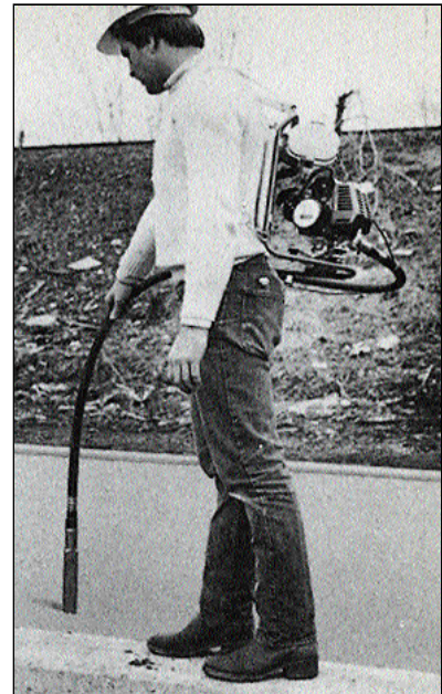
Figure 4. Backpack gasoline engine drive for this flexible shaft vibrator allows complete freedom of movement for most vibrating operations. The backpack power unit weighs 21½ pounds.
