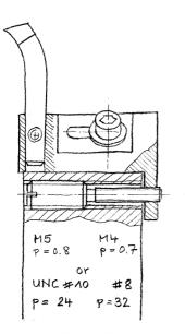
A set of 2 different threads permits a very fine adjustment of the slide. It uses the principle of the difference of 2 thread pitches. In this case a M5 with a pitch of 0.8mm and M4 with a pitch of 0.7mm.
