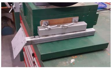
Use one of the inner tubes to make the side fixings parallel to the base.
