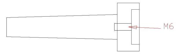
**Step 7:** Reverse the end cap, mount in a chuck and enlarge the 5 mm hole to 6 mm. Then chamfer the front and countersink the front end (to accommodate the fixing screw). I used an 11 mm drill. Drill the recess to accommodate whatever screw you will be using.
