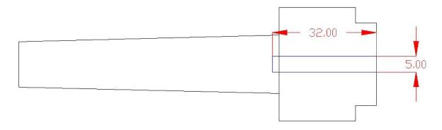
**Step 4:** Part off the front section (destined to become the cap) 11 mm from the front.
