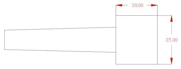
**Step 2:** Machine the front of the blank end down to 25.4 mm/1" (or for a snug fit in the slitting saw blade to be used with the arbor) for a distance of 6.5 mm.
