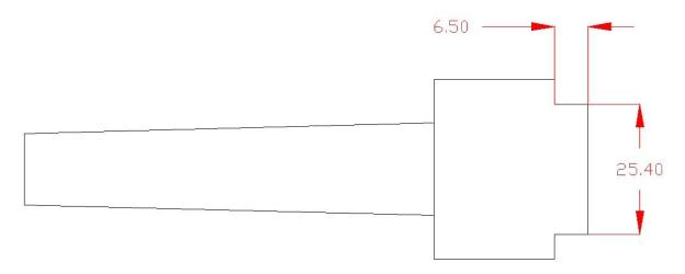
**Step 3:** Mount a 5 mm drill bit in the tailstock chuck and drill to a depth of 32 mm.
