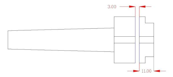
**Step 5:** Bore a 25.4 mm / 1" recess in the arbor, 5.7 mm deep. Test frequently when approaching 25.4 mm, the end cap should be a snug fit in the recess.
