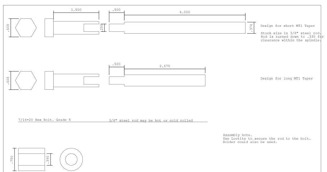
Brass or steel with 7/16-20 thread. This will be held in the lathe chuck. Use a 7/16-20 nut for a clamp.
