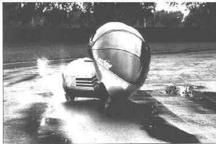
A narrow 711-mm (28-in) rear track would normally lead to poor cornering capabilities. With its leaning passenger pod, Lean Machine could negotiate 1.2-g turns.
