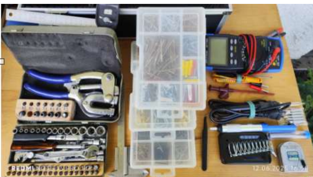
cotent 2. floor: hand punch, screws, nails, wall plugs multimeter, soldering iron and accessories
