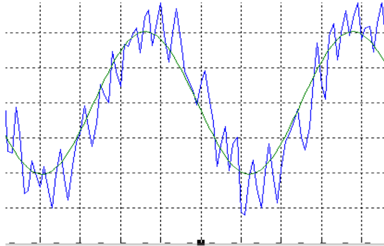
Figure 9: Induction Generator AC Output Voltage Waveform
