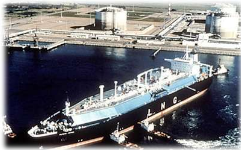
Figure 1 130 000 m 3 LNG carrier with integrated LPG→ tanks
