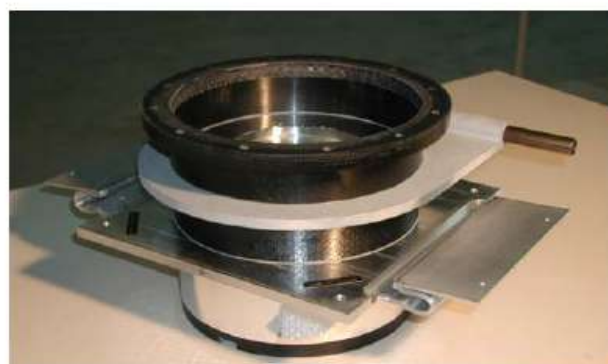
Figure 9 Non-metallic composite support post with heat intercepts for LHC superconducting magnets
