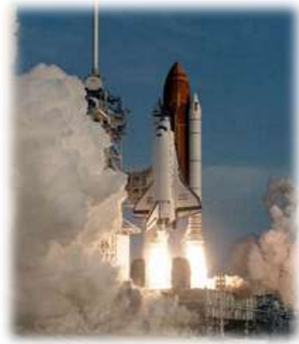
b) Space Shuttle (100 t liquid hydrogen, 600 t liquid oxygen)
