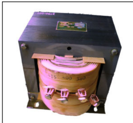
Center Tapped Transformer, 12 KVA, Input: 380/400/415 VAC, Output: -120/0/120 VAC, P/N 17790
