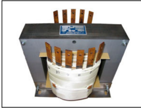
Secondary Multiple Taps Transformer, 5 KVA, Input: 240 VAC Output: 10/20/30/40/50/60/70/80/90/100 VAC, P/N 18391
