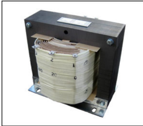
Tap Transformer, 3 KVA Input: 20/180 VAC, Output: 210/220/380 VAC P/N 18859-2
