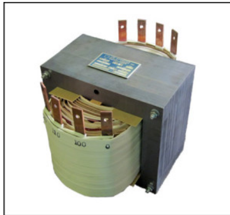
Manual Tap Changing Transformer, 10 KVA, Input: 208/220/240 VAC, Output: 100/110/120 VAC, P/N 18790
